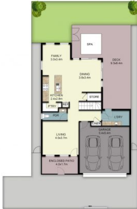
GROUND FLOOR ON SITE
